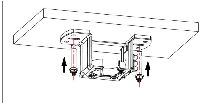
If the ceiling is made of wood or plaster, it is necessary to install 4 gravity toggles or 4 self-tapping screws to fix the bracket to the ceiling.
