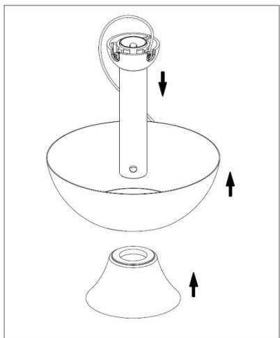
Insert the coupling rod through the canopy and the joint tube cap.
