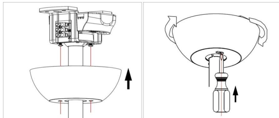
Raise the canopy and fix it by screwing it on with provided screws.
