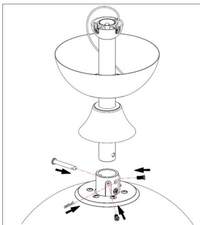
Loosen the two fixing screws of the threaded rod holder and then, place the rod in it. Align the holes of the clip with the holes in the rod holder. Fit the pin and clip.
