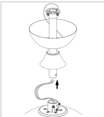
Insert the electrical wires and the earth wire through the rod.
