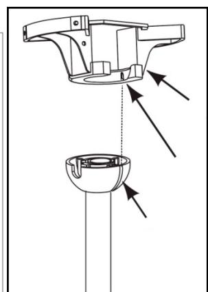
Carefully lift the fan and place the semisphere in the suspension bracket fixed to the ceiling by matching the coupling groove.
