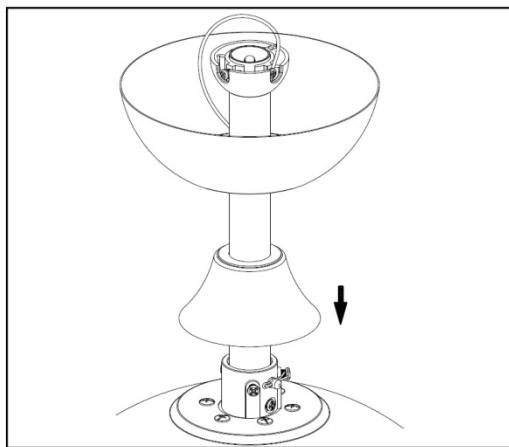
Finally, retighten the two fixing screws and lower the joint tube cap.
