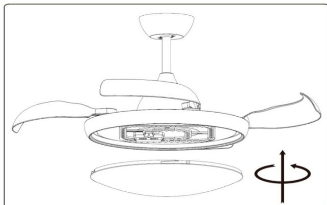
Place the diffuser on the plate and turn it clockwise.
