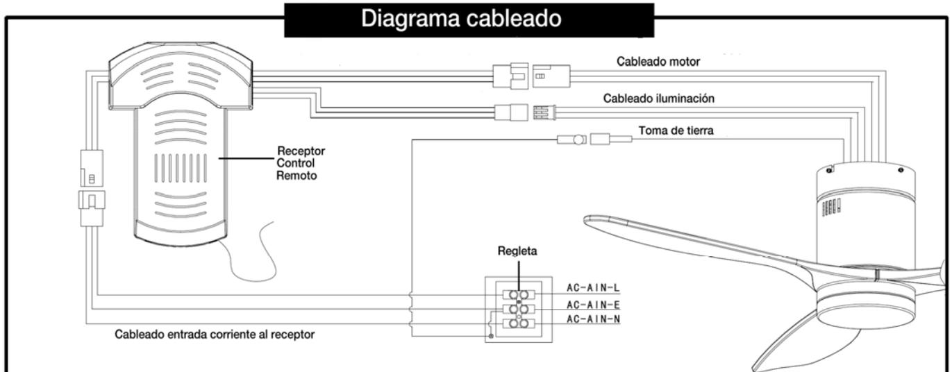
2 - Connect the power cables to the terminal strip connector.
