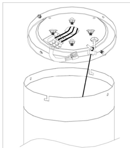
4 - Connect the fan cables to the module
