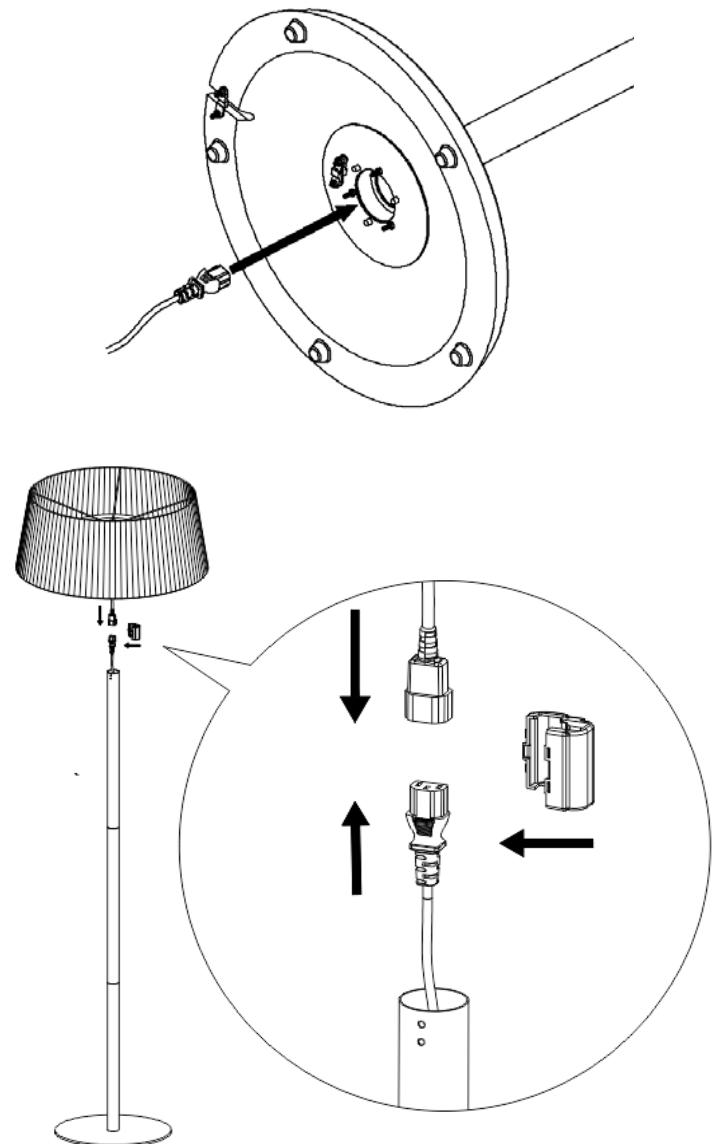
Step 5: Insert the heater head onto the top tube and fix in position using the 4\*8mm screws
