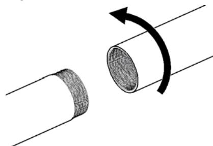
Step 3: Connect the top tube with middle tube by screwing them together (as same as Step2).
