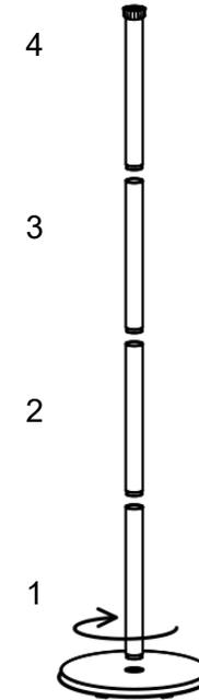
Step3: Connect the heater head with the tube by screwing them together.
